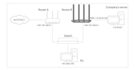
For example, in a small office, my PC can surf the internet through Router A, but I also want to visit my company's network. Now I have a switch and Router B. I connect the devices as shown in the following figure so that the physical connection between my PC and my company's server is established. To surf the internet and visit my company's
